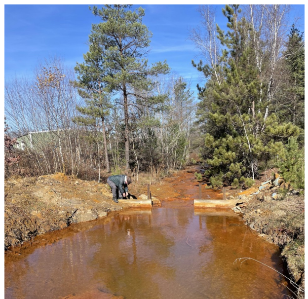
Larry Hutchinson, SCWA VP, collects needed flow data from the weir at the Reitz 4 Discharge in Central City. Photo by Tom Clark
